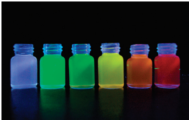
Figure 6. Fluorescence of the CdSe with different emission ( \lambda_{\text{ex}} = 365 nm).
